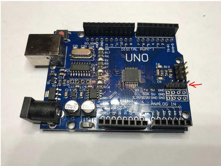
3. Cut a small length of wire for the connection between the daughter board and A5 on the Arduino UNO as well as two short lengths of wire and crimp connectors on one end for the power switch modification (if used). You can also remove the header pins for the switch on the daughter board and solder wires directly to board.
