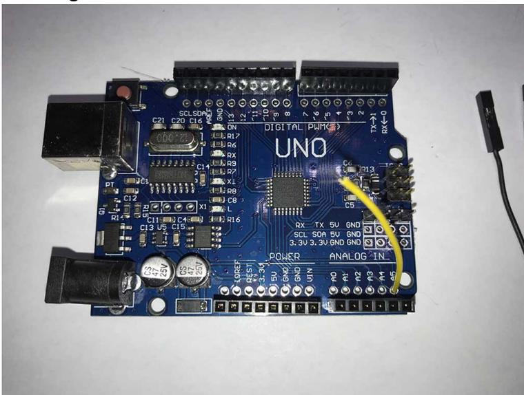
5. Solder the short wire to the A5 Through Hole on the daughter board and slide daughter board over the header pins on the Arduino UNO. You may have to bend the pins on the header you attached above as the alignment is not perfect, but they will fit if a small force is used.
