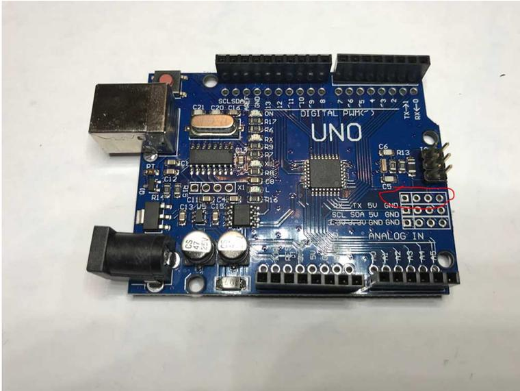
2. Solder a 4-pin header into the holes.
